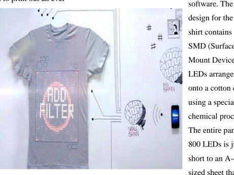
design for the Tshirt contains SMD (Surface Mount Devices) LEDs arranged onto a cotton cloth using a special chemical process. The entire panel of 800 LEDs is just short to an A-4 sized sheet that
